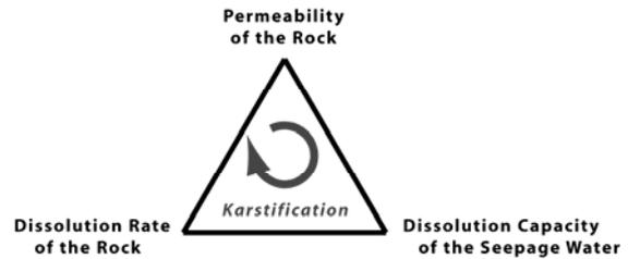
Fig. 1: The process of karstification is a positive feedback loop controlled by factors controlling the rock permeability, dissolution rate and dissolution capacity of the seepage water.
